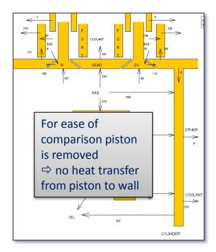
Gas temperatures and HTC's for GT Customized FE model and STAR-CCM+ model are identical.
