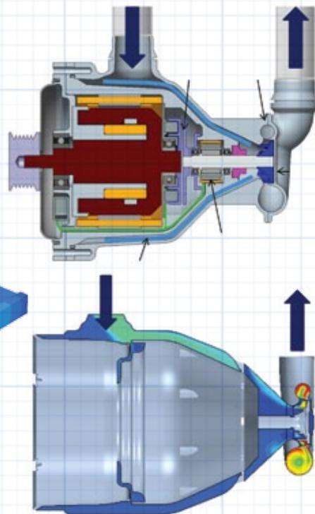
**TOP** Combined generator/coolant pump from IGEL AG
